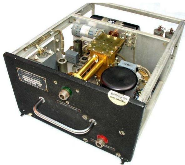
In the 15.5 x 26.5 x 33 cm case, the transmitter is on the right. The big black dome is a centrifugal speed controlled dc motor, which drives a variable capacitor for frequency modulation. The gold plated pipes in the middle are the receiver input circuit, matching the antenna to the balanced mixer in a gold plated box.
