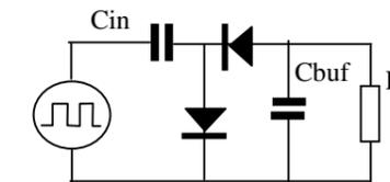
$C_{buf}$  must have a low impedance, so the output voltage remains small compared to E.
