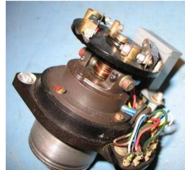
In fact, there are two contacts, one opening at 800rpm, the other at 4000 rpm. Which one controls the speed is selected in the cockpit. The lower speed is used for high altitude, with a useful range of 0-5000 feet, the high speed for the low altitude range of 0-1000 feet. The measured altitude is proportional with the speed of this motor, so the gap in the centrifugal contacts is critical and probably needed frequent cleaning and adjustment.
