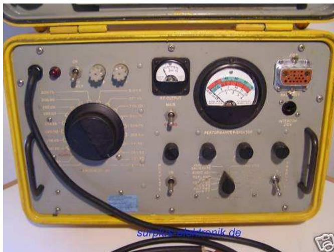
Radio Test Set; manufactured by Systems Development; used with AN/ARC-34
