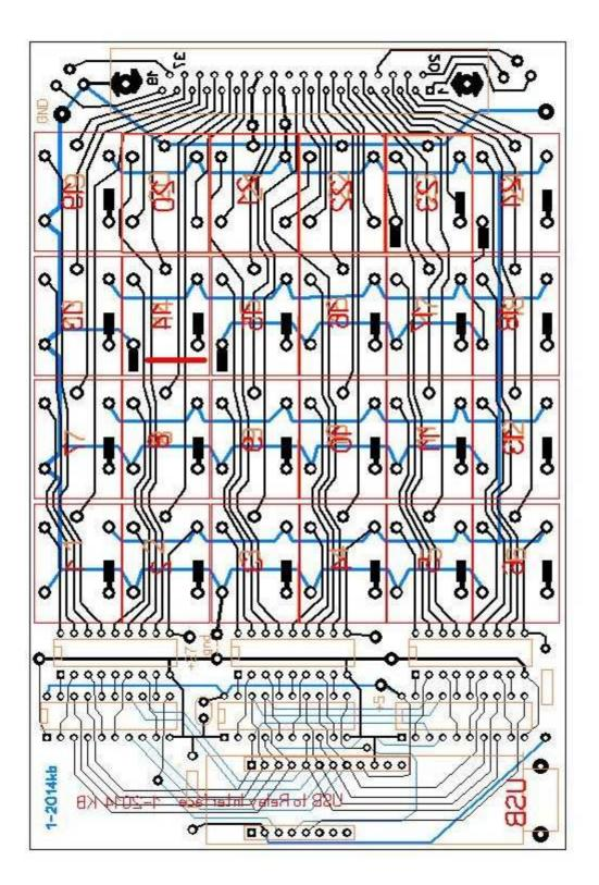
Relay Interface Board, *component side* A few (empty) boards are available - dual side, thru plated, with on both side solder masks and silk screen
