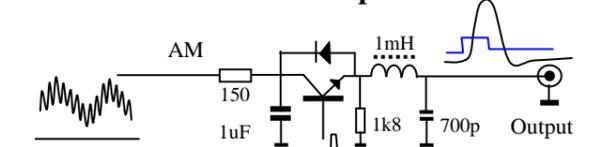
The modulator transistor switches the AM wave to the output LC circuit for approx. 3μs. During this time, the output capacitor is charged to twice the AM voltage ( 18V max).
