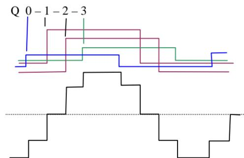
Each stepped wave is filtered to a sinewave with 1% distortion in a second order filter. The sinewaves are added to get the typical TACAN envelope.
