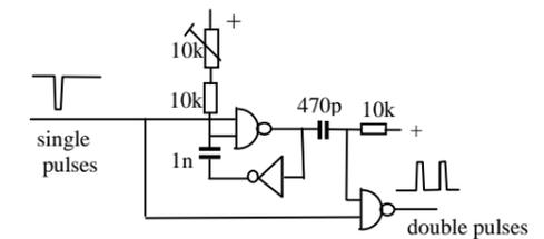
The twin output pulses still have slightly different widths, but these are all made equal in the output cosine pulse shaper.
