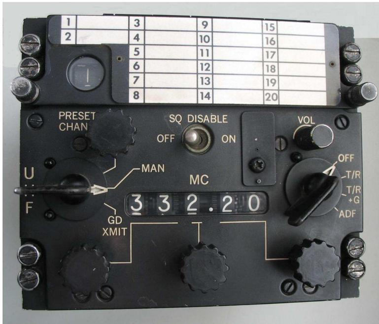
Compared to the ARC34 control, a squelch disable was added, and readout of the manual frequency is far better.
