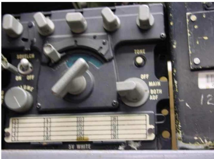
Maybe this control was also used for the ARC34C. It has a fifth knob for the 50kHz channel separation.
