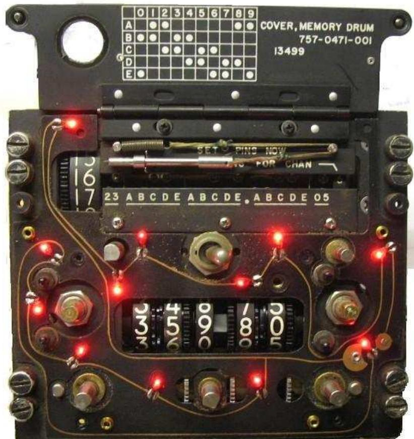
C-6287/ARC-51BX with front cover removed. The lamps are in two strings of 6 each.
