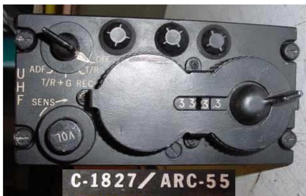
**C-1827/ ARC-55** is a simple control without preset channels.
