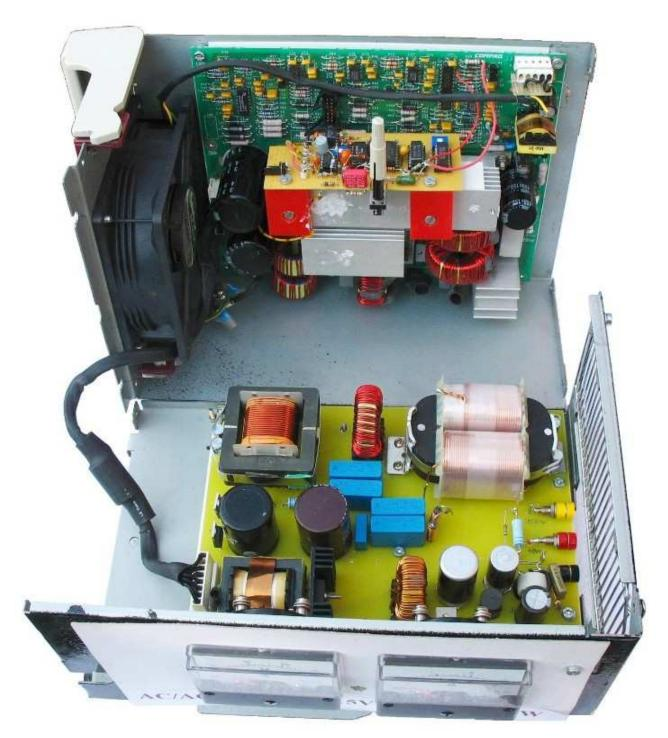
Finally, a C-core transformer with 1:1 turns ratio provides isolation between the mains and the 400Hz output. Behind the meters are some components that were salvaged from the original PS4060 secondary board to provide a 24Vdc/3A output, needed as well by most avionics .
