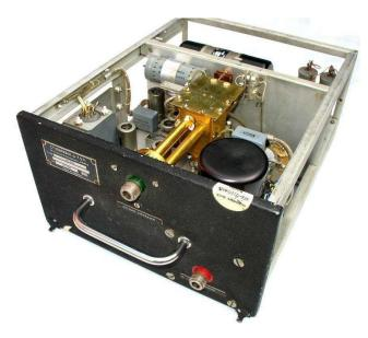
In the  $15.5 \ge 26.5 \ge 33$  cm case, the transmitter is on the right. The big black dome is a centrifugal speed controlled dc motor, which drives a variable capacitor for frequency modulation. The gold plated pipes in the middle are the receiver input circuit, matching the antenna to the balanced mixer in a gold plated box.
