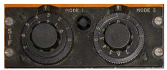
C-1128/APX-25 Is connected to the KY95 coder unit.
