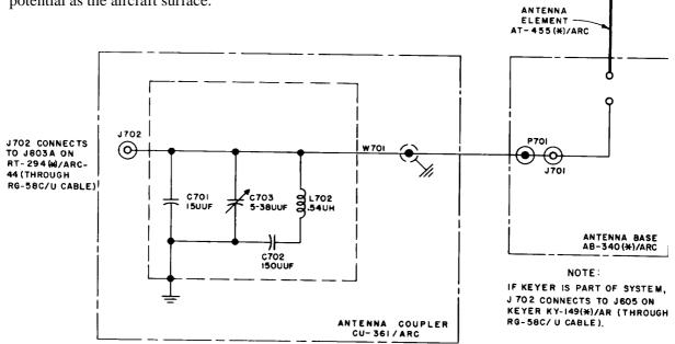
Figure 2-26. Antenna AT-454(•)/ARC, schematic
