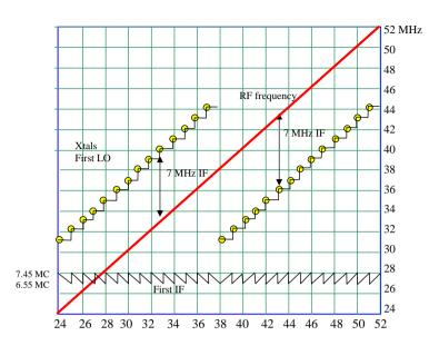
The first local oscillator frequency is set by one of 14 Xtals, mounted on a turret. The turret makes two complete revolutions, the first with the LO frequency *above* the signal frequency, the second turn with the LO frequency *below* the signal frequency. Because the frequency step halfway is 14MHz, this implies a first intermediate frequency of 7MHz.
