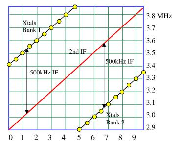
Horizontal in this plot is the position of the 0.1MHz digit on the control panel. Vertical are the 20 Xtal frequencies of the third LO (vellow dots) and the permeability tuning of the second IF bandpass filter (red line), all in MHz.
