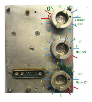
The various tuned filters and Xtal oscillators realize the MHz,- and sub MHz dials at the cockpit control panel. Three relays reconnect the IF filters in transmit mode, in order to add the local oscillator frequencies to compose the carrier frequency. To make the transmit frequency equal to the receive frequency, the first, second and third LO frequencies shall be added to the last IF frequency of 500kHz.
