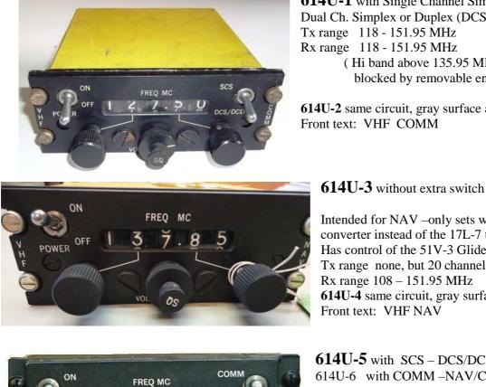
**614U-1** with Single Channel Simplex(SCS) or Dual Ch. Simplex or Duplex (DCS/DCD) switch. Tx range 118 - 151.95 MHz Rx range 118 - 151.95 MHz (Hi band above 135.95 MHz can be blocked by removable end stop )
