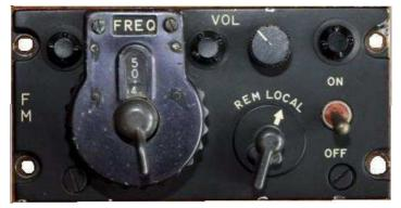
The SB-327 / AR selects the frequency from 24.0-51.9 MHz in 100kHz steps is a total of 280 channels.
