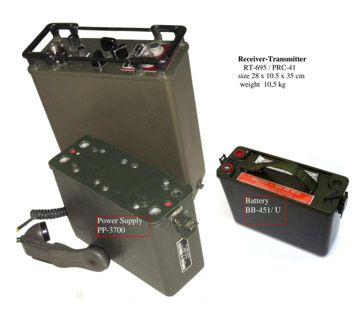
Either the battery or the ac power supply can be attached to the RT695. Both have the same size (28 x 10.5 x 19 cm) and weight (7.5 kg) The battery must be charged with a special charger, not this PP-3700
