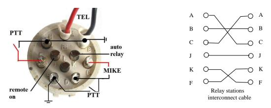
The basic PRC-41 has two of these 10-way connectors, all pins are connected in parallel.
