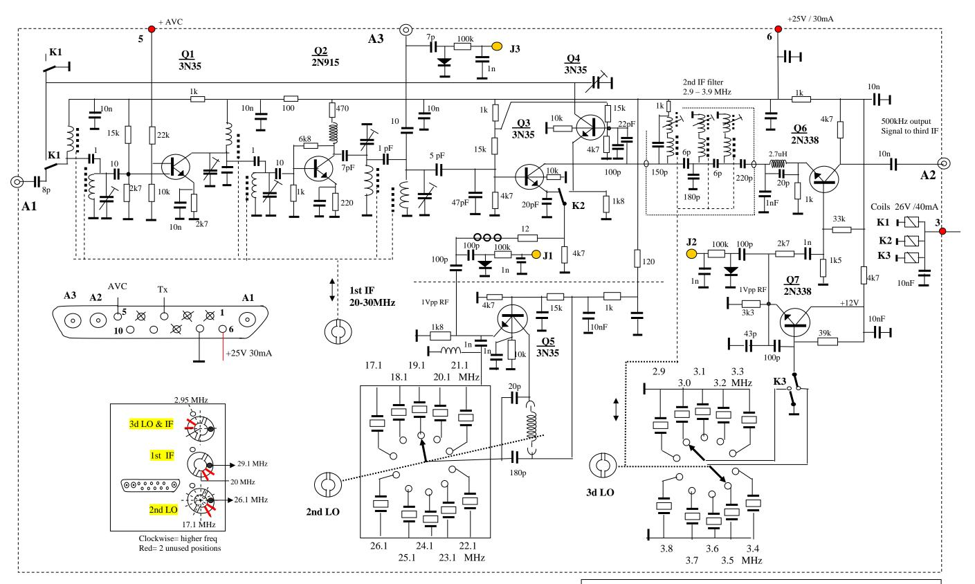
PRC-41 First and second IF amplifier (A2)  $_{3 \text{ nov } 2017 \text{ kb}}$
