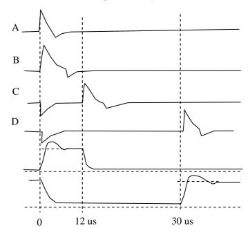
**Pulse D** checks if the received pulse is longer than 30us, to produce a 1 kHz tone during a dot or dash of the beacon identifier (ID). Eureka beacons normaly respond with short (5us) pulses. However, every few minutes a beacon ID is transmitted as a two-letter morse code by widening the response pulse to 33us during the dots and dashes.
