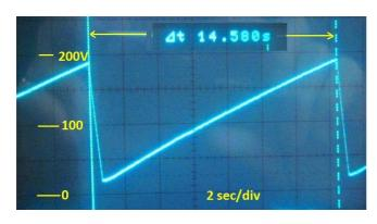
The 200nm search cycle takes 14 sec with a 0.5mA range meter connected (and 150k extra series resistor). Without meter the cycle takes only 12 sec (?!)
