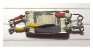
It is nearly impossible to re-wind the original transformer because the ferrite core is brittle, and glued inside the bobbin.
