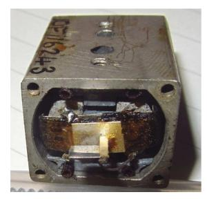
attached which is the moving contact. To handle the low contact pressure, both the vane and the contacts are made of 80% platinum, 20% iridium.
