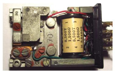
The sensitivity of this relay is remarkable: 0.12mA x 0.4V with both coils in series is 0.05 mW!!
