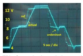
The position of the tuning elements is measured with a potmeter, producing a voltage between 1.7V (approx. 240 MHz) and 22V (approx. 193 MHz). The channel selection in the control panel provides a voltage in the same range. When the difference between these two voltages is more than 0.1V, the motor runs either forward or backwards.
