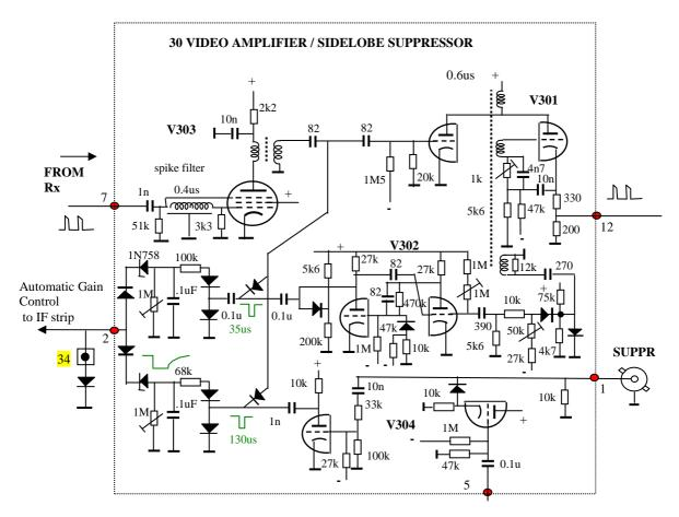
A blocking oscillator shapes the received pulses to 0.6us wide pulses with fixed amplitude. The circuitry around V302 detects the new SLS pulse if present, at 2us after the first pulse If present, a 35us pulse blocks the third pulses, as well as the IF amplifier.
